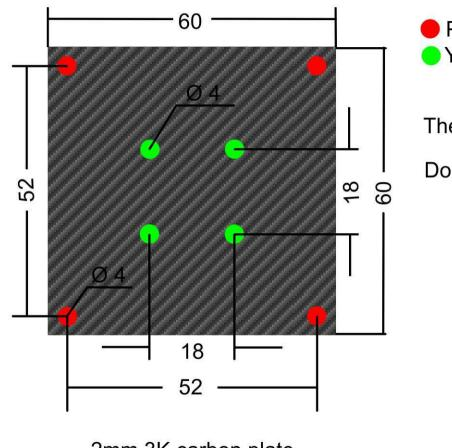
Plate mounting holesYAW-motor mounting holes
