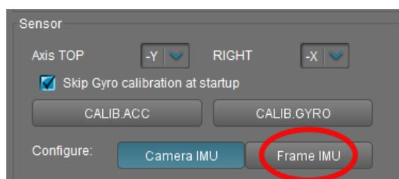
If the second IMU is connected properly, this button becomes active. It means that all IMU settings now affect on the frame IMU. Change sensor orientation (axis TOP, RIGHT) and write setting to the board, if necessary (board will be restarted). After restart, calibrate the accelerometer and gyroscope like you did it for the main IMU. For the accelerometer, you can do simple calibration or extended 6-point calibration.
